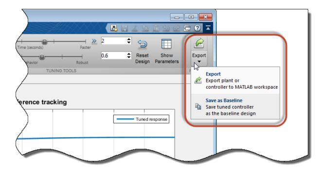
When you do so, the current Tuned response becomes the Baseline response. Further adjustment of the current design creates a new Tuned response line.
